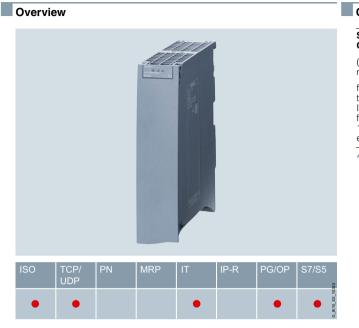
The SIMATIC CP 1543-1 communications processor securely connects the new SIMATIC S7-1500 controller to Industrial Ethernet networks. By combining a variety of security features such as an SPI (Stateful Packet Inspection) firewall, VPN and data encryption protocols such as FTPS and SNMPv3, the communications processor protects individual S7-1500 stations or even entire automation cells against unauthorized access.
