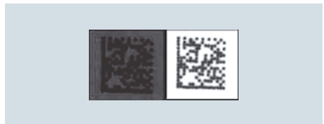
Very little or non-uniform contrast in the marking
