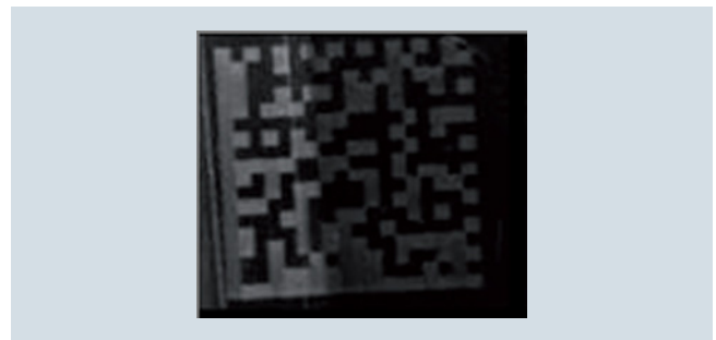
Very little or non-uniform contrast in the marking
