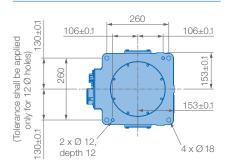
Mounting options: Floor, ceiling, wall, tilt\* Protection class: IP67
