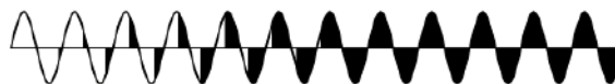
Soft start switching in case control signal has been missing in the previous 5 seconds
