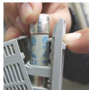
4. Pressing downwards the fuse-holding clip to insert or remove the fuse
