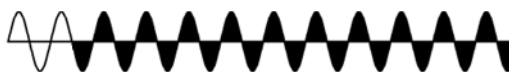
No soft starting in case control signal has been present in the previous 5 seconds
