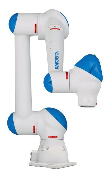
MOTOMAN HC10 is a 6 axes human-collaborative robot with a payload of 10 kg. Operator's safety is assured by a Power and Force Limit technology that stops the robot in case of contact with an operator.
