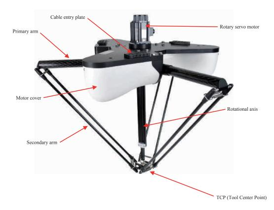
The CR\_UGD4\_XL robot consists of three radially placed axis which give the TCP freedom to move in three directions, X, Y and Z. An optional fourth axis can take care of the rotation, Rz, of the TCP.
