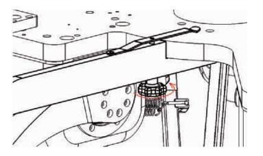
• Now tighten the star nut until the tool is fixed
